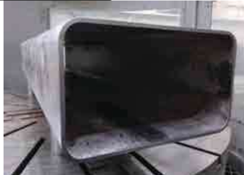
Bend a steel plate into a rectangular shape and form a rectangular pipe by welding the butted seam using electron beam welding (EBW)
